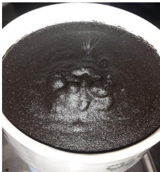
Figure 48: HTL crude produced from black liquor (Source: VTT)
