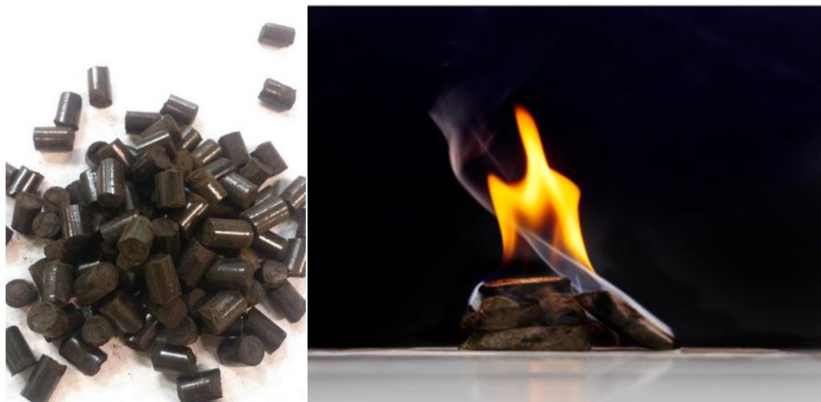
Figure 45: Biocoal pellets and hydrochar produced with C-Green's HTC-process (Source: C-Green)
