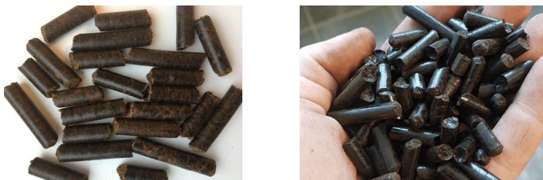
Figure 9: Thermally treated biomass pellets. Left: steam exploded Arbacore wood pellets (Source: Arbaflame). Right: torrefied wood pellets (Source: Yilkins)
