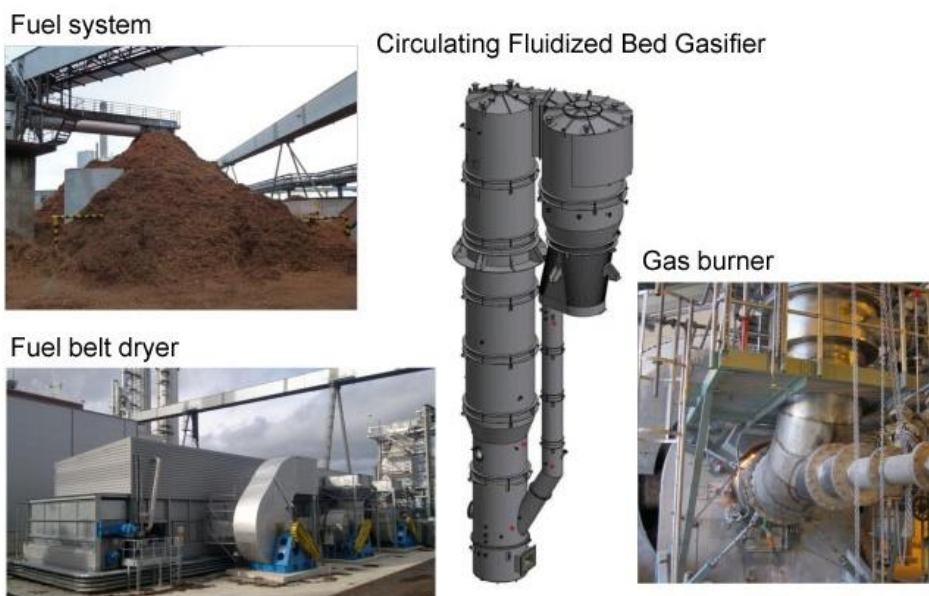
Figure 50: Components of a gasification plant (Know pulp, 2019)
