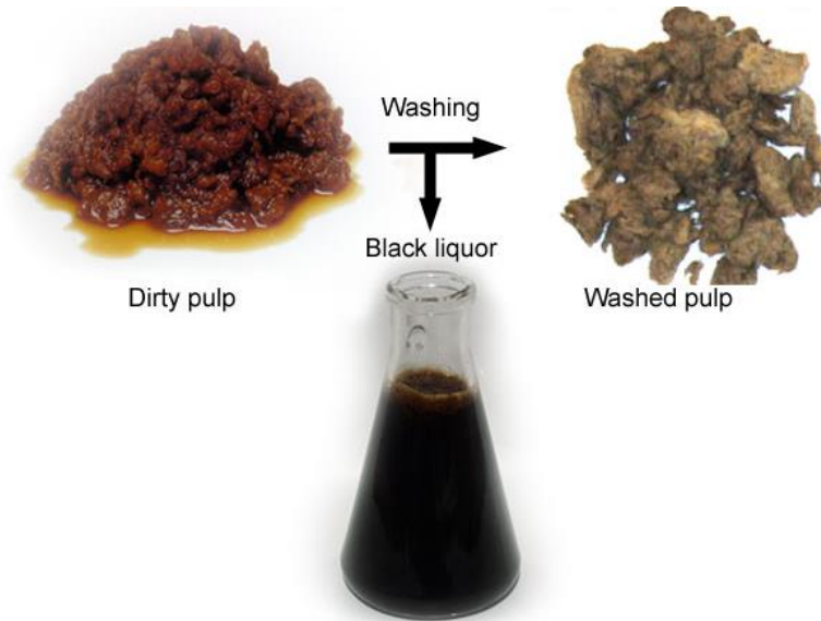
Figure 37: Washing of dirty pulp produces black liquor and washed pulp (KnowPulp, 2019)
