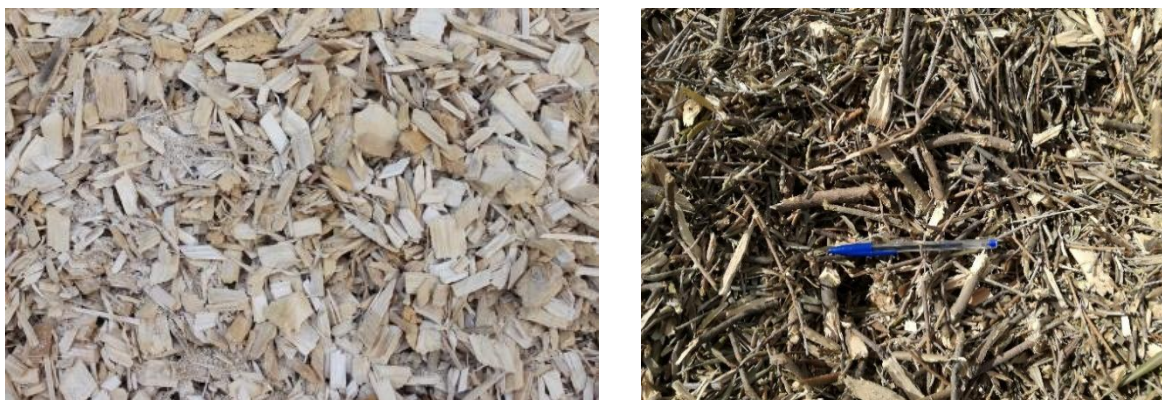
Figure 8: Left - wood chips from forest (Source: Rutz D.), Right – hog fuel from olive tree prunings (Source: Karampinis E.)
